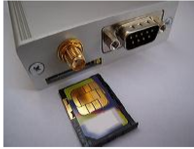
The way to install the SIM card
