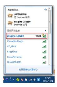
User can use a PC to connect to this WiFi network. The PC will get an IP address 10.130.1.xxx and the LPS8N has the default IP 10.130.1.1
