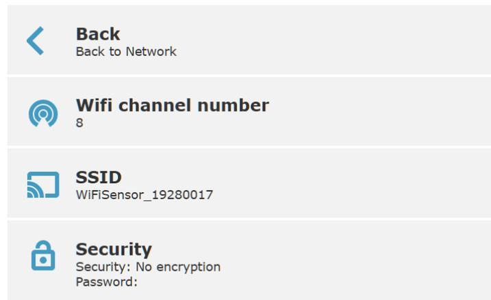
At the AP mode Wi-Fi sensor have own DHCP and DNS server. Network parameters are stated below (parameters are not configurable from web). When Wi-Fi sensor at AP mode is configured from cell phone, it is recommended to deactivate mobile data.
