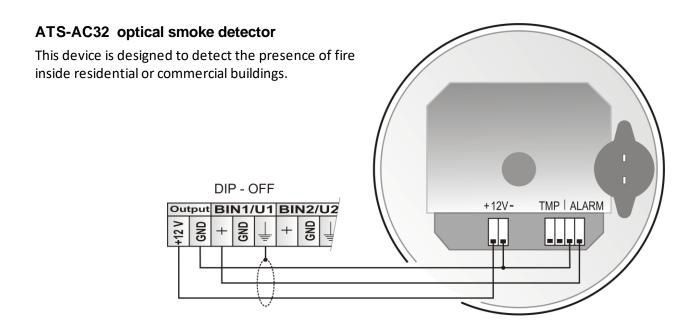
**Notice:** The connecting cables should be located as far as possible from the potential interference sources. The cable shield connect to "Shield" terminal of regulator only.
