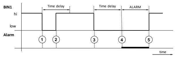
A figure shows a simple example. Binary input 1 is configured to send an e-mail if input change state from high to low (lower edge). At point 1 a binary input was opened. Because at point 2 input was closed before the time delay expired, alarm was not set. At point 3 was input opened again. At point 4 the time delay expires and at this moment e-mail, SNMP traps are sent. The alarm lasted to point 5, where the input was closed.
