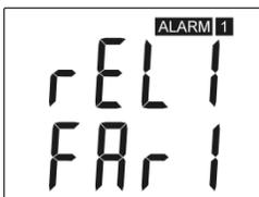
FAR0 – „far condition 0“: after device’s power on the relay is open
