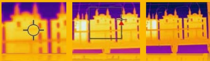
The LCD display resolution may well be 640 x 480, or capable of displaying 307,200 pixels (640 multiplied by 480) of image content. But if the IR detector pixel resolution (the “feed”), is only 160 x 120 or 19,200 pixels, then the display resolution capacity is irrelevant.
